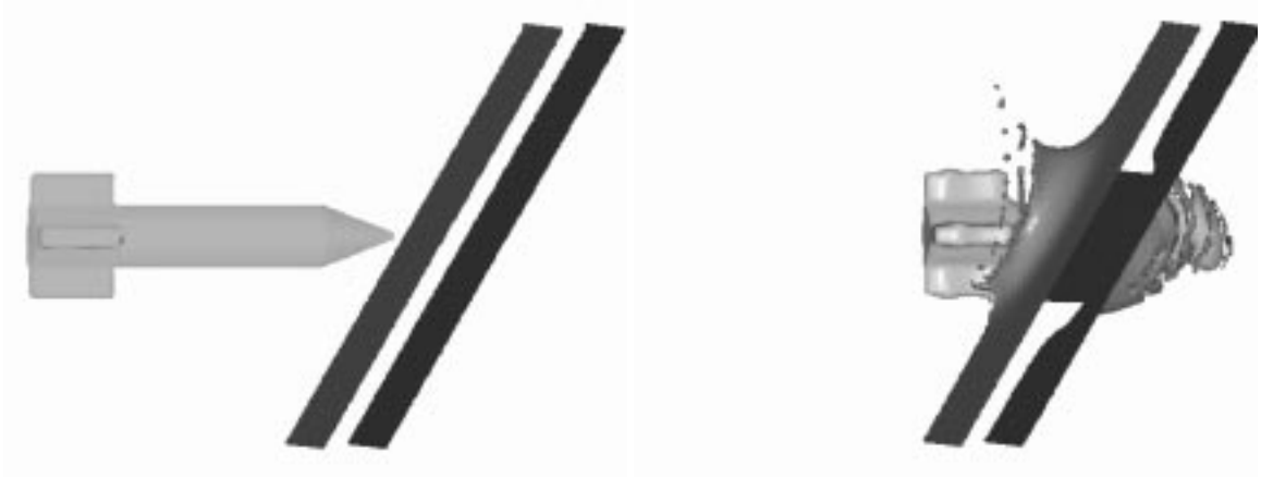
Figure 6. Simulation of a finned tungsten projectile obliquely impacting a stainless steel plate (hydrodynamic constitutive model).
